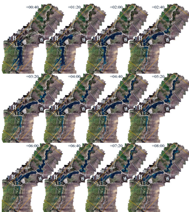
Figure 7 – Results of flood modeling due to the break of the Voroshilov Reservoir dam
